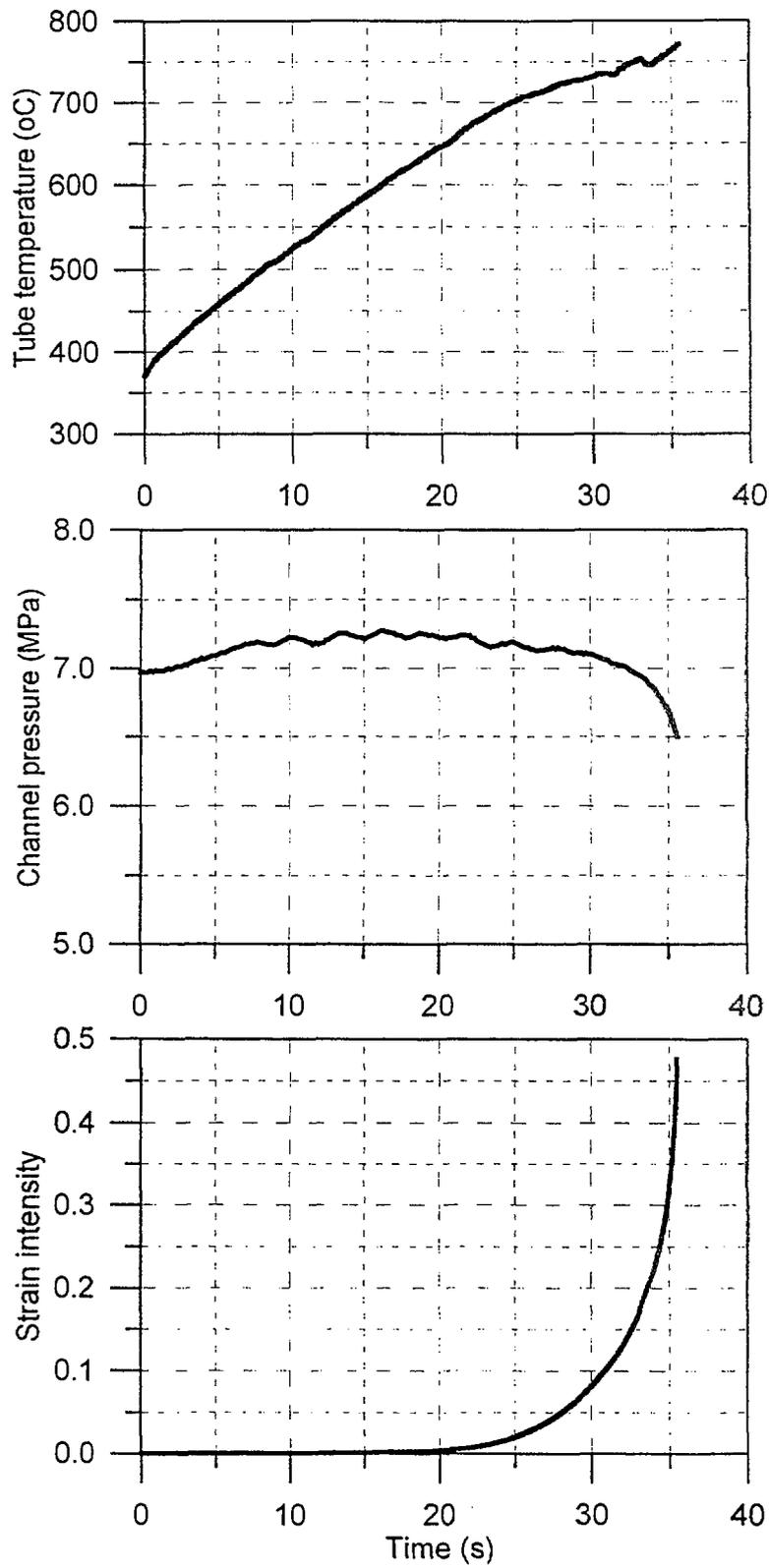
FIG. 15. Test with section of regular RBMK pressure tube without graphite blocks.
