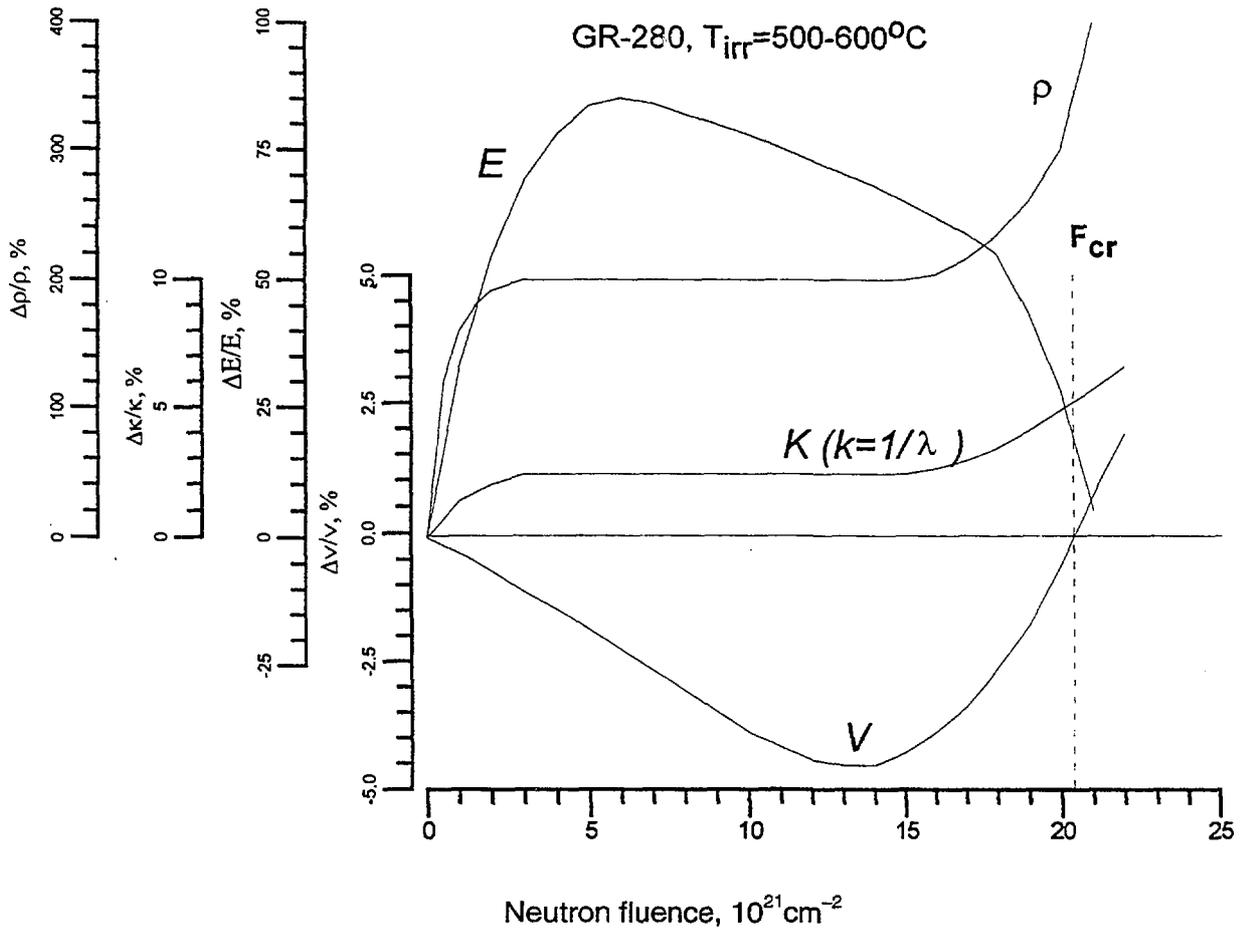
FIG.8. Determination of neutron fluence critical values for graphite physical properties changes (*V*-volume, *E*-elastic modulus, *k*-thermal resistivity,  $\rho$ -electrical resistance).
