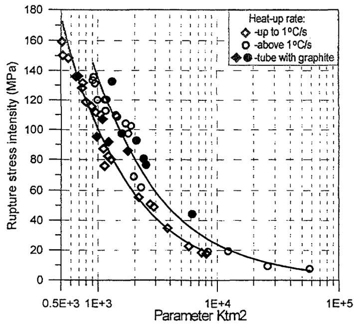
FIG. 13. Pressure tube rupture stress intensity versus parameter  $K_{tm2}$ .
