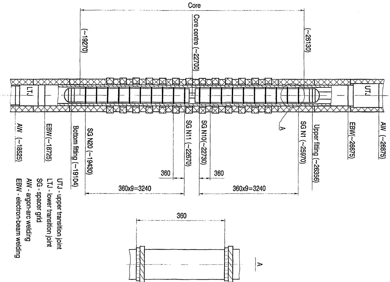
FIG. 3. Fuel channel and fuel assembly components.
