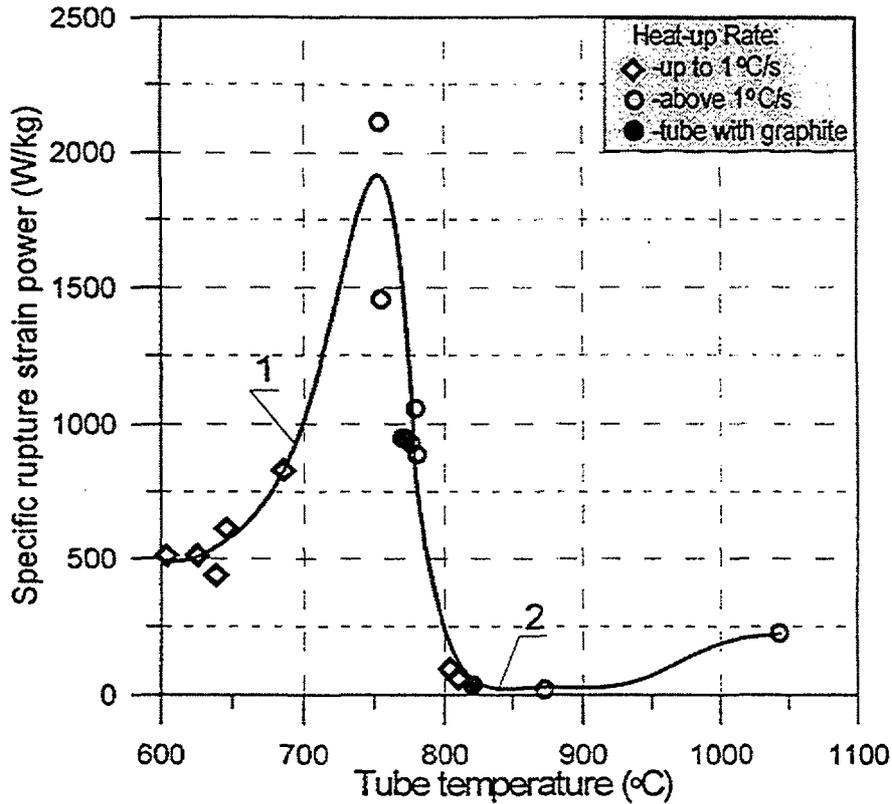
FIG. 14. Pressure tube rupture strain power versus pressure tube temperature.
