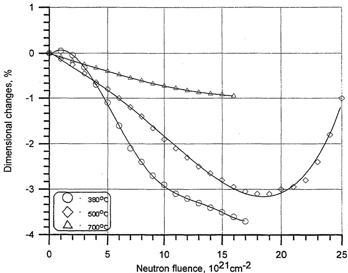
FIG.7. Relative dimensional change of reactor graphite samples (GR-280) in axial direction.
