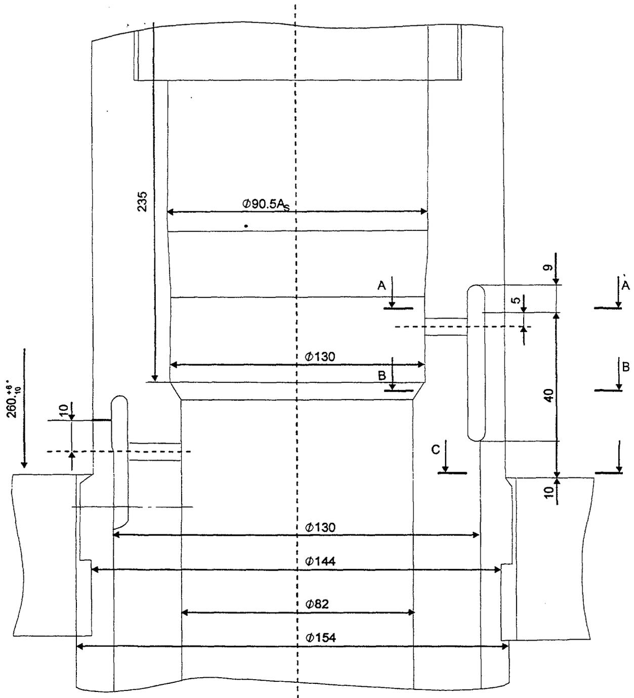
FIG.17. Upper standpipe to fuel channel plug housing weld; original and after repair configurations.
