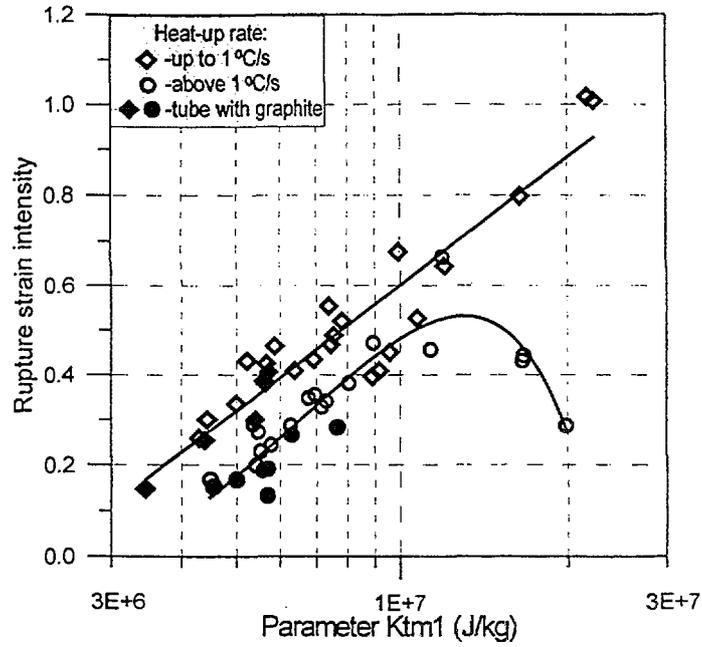
FIG. 12. Pressure tube rupture strain intensity versus parameter  $K_{tm1}$ .
