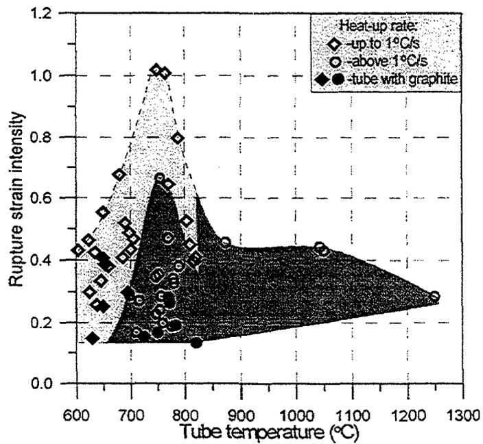
FIG. 11. Pressure tube rupture strain intensity versus pressure tube temperature.
