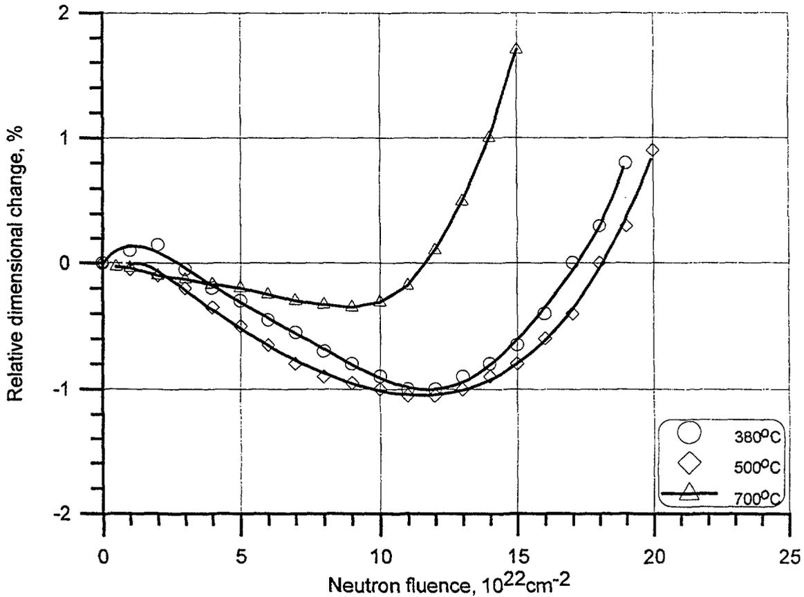
FIG. 6. Relative dimensional change of reactor graphite samples (GR-280) in radial direction.
