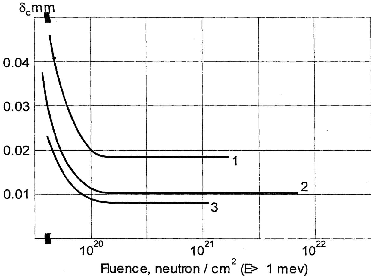
FIG.4. The effect of neutron irradiation on the fracture toughness of RBMK pressure tubes in terms of  $\delta_C$ ,  $T=300^\circ\text{C}$ , 1-TMO 2, 2-annealed, 3-TMO 1).
